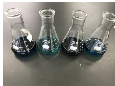
Figure 9 : Liquid treated by reacting Zn, Sn, Mg, and Fe copper-supported powders (from right to left)
